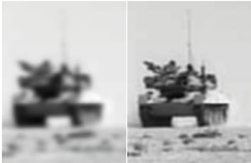
Pixion-method deblurring. When viewing over long distances at high magnification, atmospheric turbulence warps and blurs the image.
