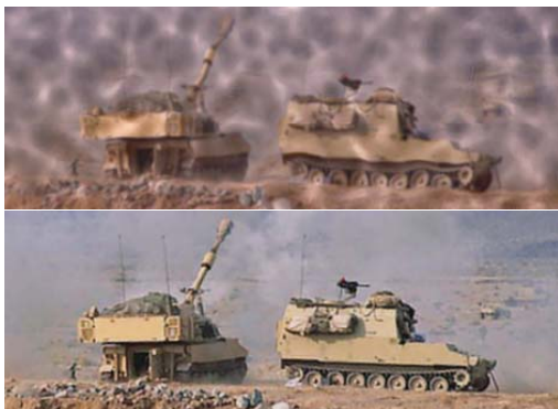
Performance that will be achieved by image-dewarping hardware being developed for the Army.
